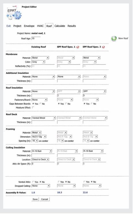
The Davis Energy Calculator was used to estimate the energy performance of a ccSPF roofing system and a metal roof deck with fiberglass insulation on the underside of the deck. The batt insulation provided negligible insulation value for the conditioned warehouse, while the ccSPF roofing system provided a higher R-value performance than the rated R-value of the foam.
