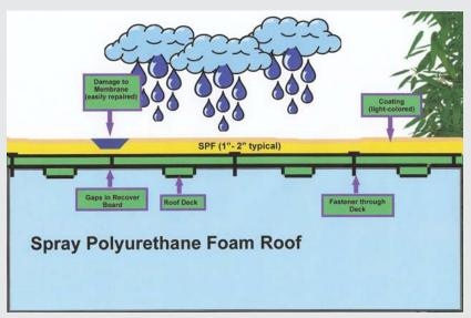
As these illustrations show, the closed-cell foam of ccSPF roofing does not allow water to travel laterally even if the foam surface is damaged. Repairs can be easily made with sealant or foam packs.
